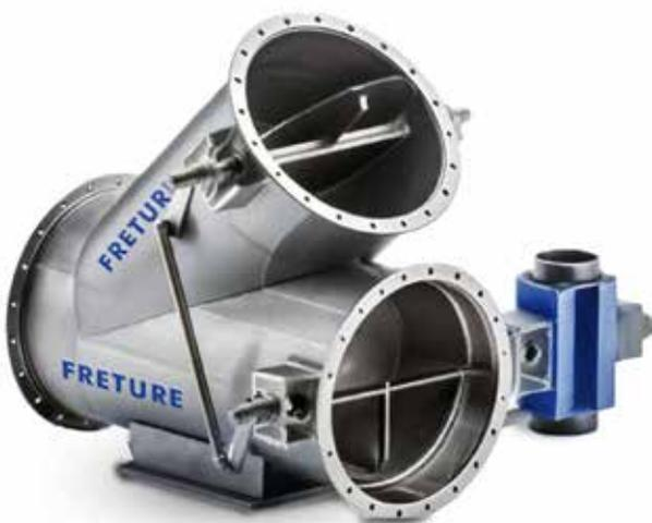
Freture Techno's Diverter dampers are key for directing airflow or gas in industrial systems. Available in round, square, and rectangular configurations, they are made from stainless steel or painted carbon steel for durability. With a shutoff capability up to 99% and various seal options like tadpole, metal seat, and swing-thru, they ensure tight control.
